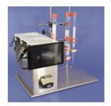
Simple to use, low-pressure FPLC chromatograph based on UV detector and peristaltic pumps (max. pressure level about 4 bar)
