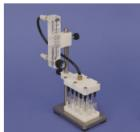
Evaporation under nitrogen and optional heating block
